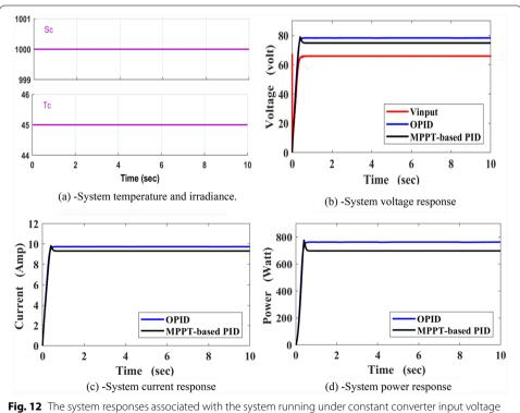
**Fig. 12** The system responses associated with the system running under constant converter input voltage (constant array temperature and irradiance)
