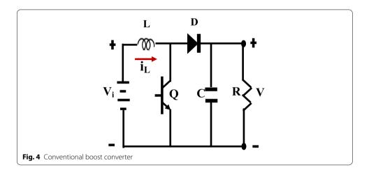
$$\begin{cases} \frac{\mathrm{d}i_L}{\mathrm{d}t} = \frac{1}{L}(V_{\mathrm{in}}) \\ \frac{\mathrm{d}v_0}{\mathrm{d}t} = \frac{1}{C}(-\frac{v_0}{R}) \end{cases}, \quad 0 < t < \mathrm{d}T, \ \underline{O} : \ \mathrm{ON}$$
