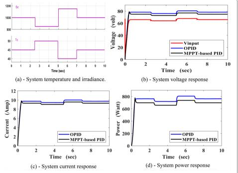
**Fig. 13** The system responses associated with the system running under variable converter input voltage (variable array temperature and irradiance)
