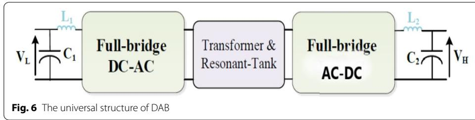
Fig. 6 The universal structure of DAB
