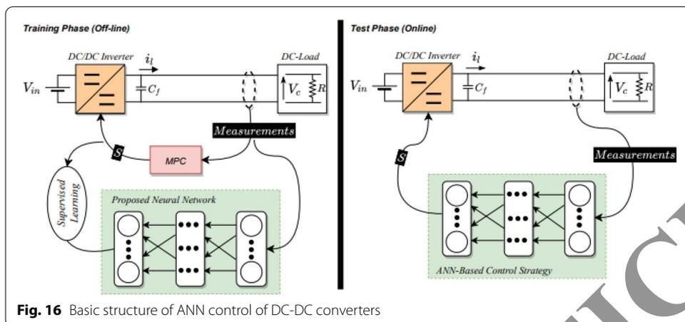
Fig. 16 Basic structure of ANN control of DC-DC converters
