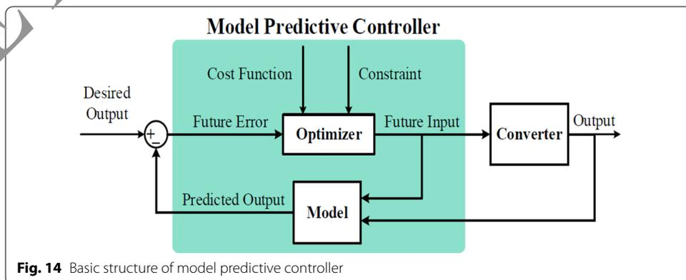
Fig. 14 Basic structure of model predictive controller
