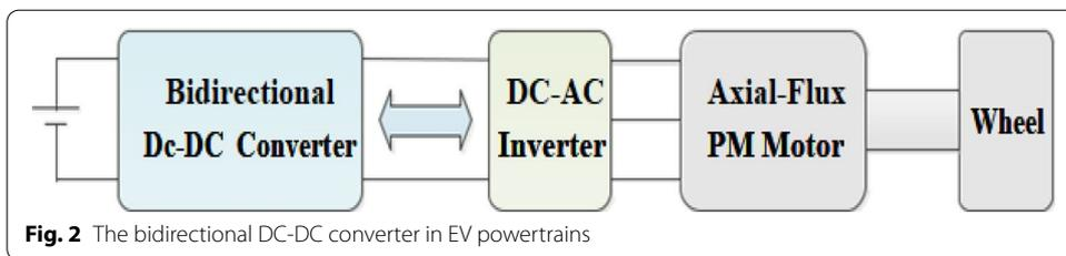
Fig. 2 The bidirectional DC-DC converter in EV powertrains
