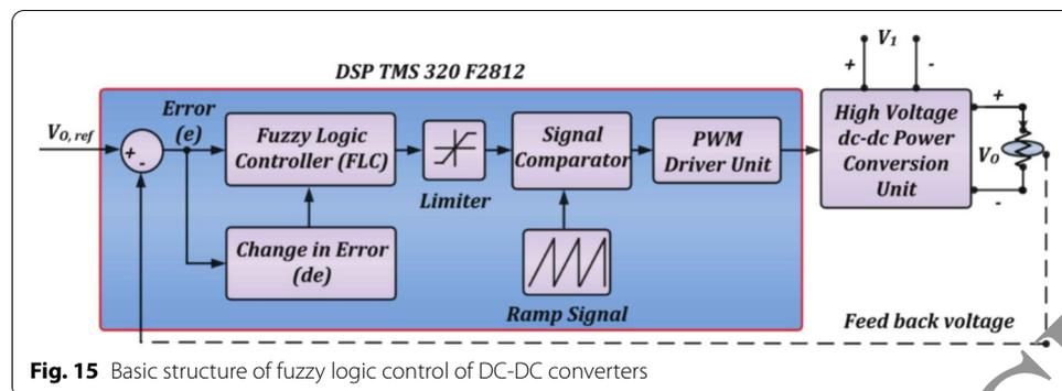
**Fig. 15** Basic structure of fuzzy logic control of DC-DC converters
