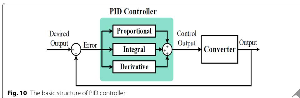
**Fig. 10** The basic structure of PID controller
