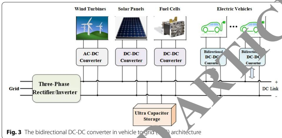
Fig. 3 The bidirectional DC-DC converter in vehicle to grid (V2G) architecture
