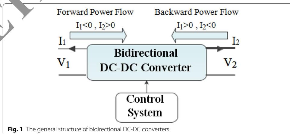
**Fig. 1** The general structure of bidirectional DC-DC converters
