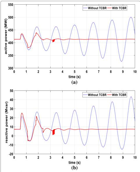
**Fig. 5** Power flow responses to the small disturbance with and without the TCBRs interventions, **a** inter-area active power flow, **b** inter-area reactive power flow
