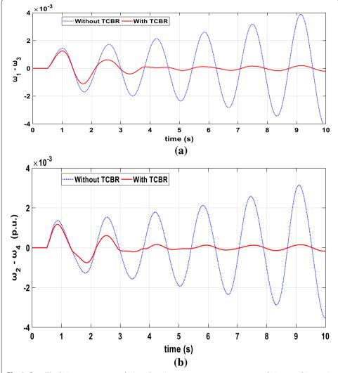
**Fig. 9** Case (2) relative generator speeds time-domain responses, **a** outer generators relative speed ( $\omega_1 - \omega_3$ ) in (p.u.), **b** inner generators relative speed ( $\omega_2 - \omega_4$ ) in (p.u.)
