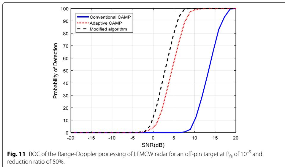
modified algorithm compared with both the traditional and adaptive CAMP, as illustrated in Fig. (11). This is due to the modification in the threshold calculation of the CA-CFAR processor of the reconstruction algorithm.
