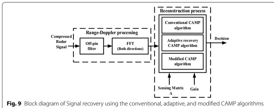
**Fig. 9** Block diagram of Signal recovery using the conventional, adaptive, and modified CAMP algorithms
