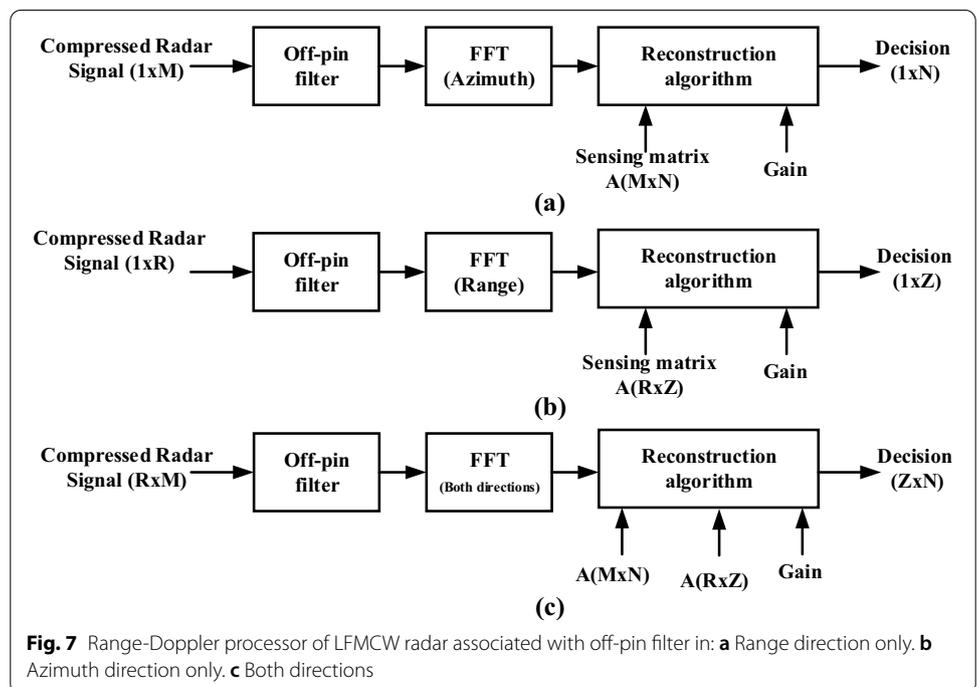
**Fig. 7** Range-Doppler processor of LFMCW radar associated with off-pin filter in: **a** Range direction only. **b** Azimuth direction only. **c** Both directions
